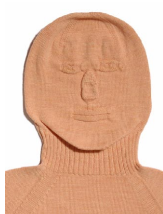
5 Final sample. Smooth shaping and minimal finish possible with the addition of 2 x 2 rib to give more texture and achieve shaping for neck and shoulders.
