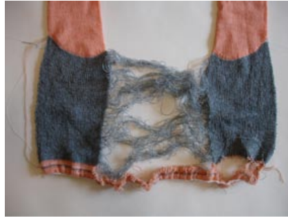
2 The knitting process starts at the toe ends. Long waste yarn is needed to get beyond the Takedown Rollers. It is necessary to remove the grey waste yarn from the toes (sock ends) when the knitting comes off the machine.
