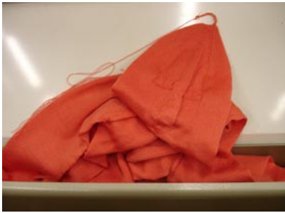
1 The bodies are knitted feet first ending with the top of the head. They fall from the machine fully knitted.
