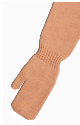
9 The hand/mitten end shaping was achieved through the use of the Drawstring Edge. Wrist shaping was achieved through the addition of 2 x 2 rib.
