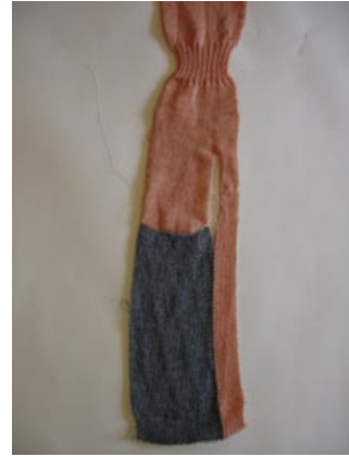
3 The waste yarn on the hands (mitten ends and thumbs) needs to be right length to hit the sub rollers before starting to knit the hands in main yarn. It is necessary to remove the grey waste yarn when the knitting comes off the machine.
