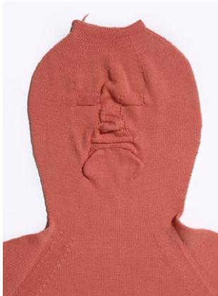
4 First full-size sample. Trying to shape top of head without having noticeable fully fashioning marks. It was not possible to get the amount of shaping needed through this method.
