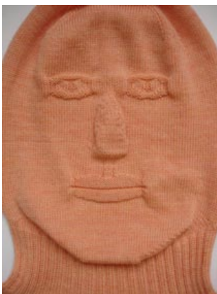
7 Final sample. Achieving three-dimensional detail in face whilst maintaining knitted fabric quality through use of partial knitting (flashage) and interlock (birdseye).
